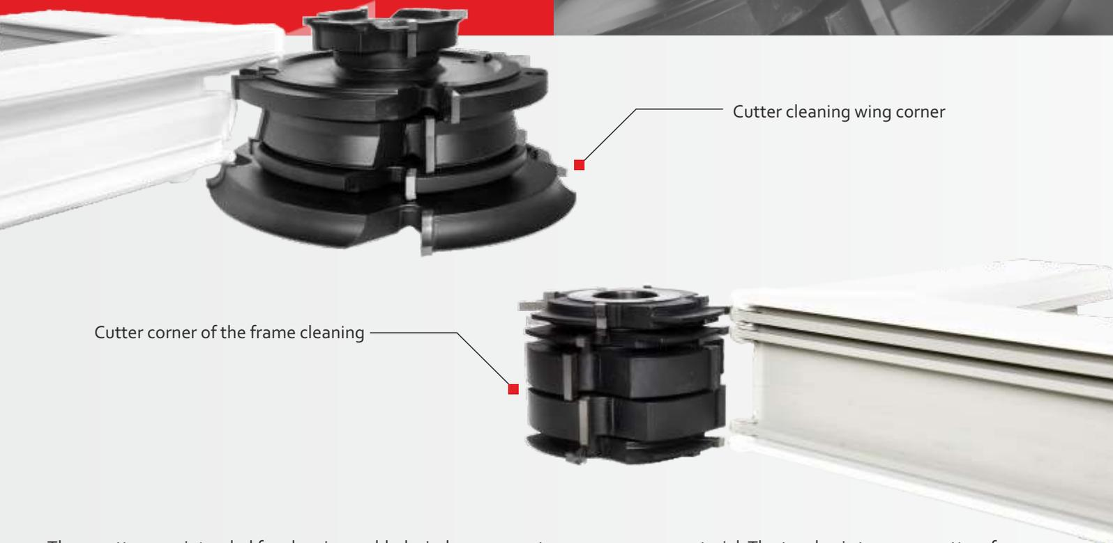
These cutters are intended for cleaning welded window corners to remove excess material. The two basic types are cutters for frames and cutters for sashes. The blades are made from carbides specially selected for milling of PVC. We use carbides from the best global suppliers only.
