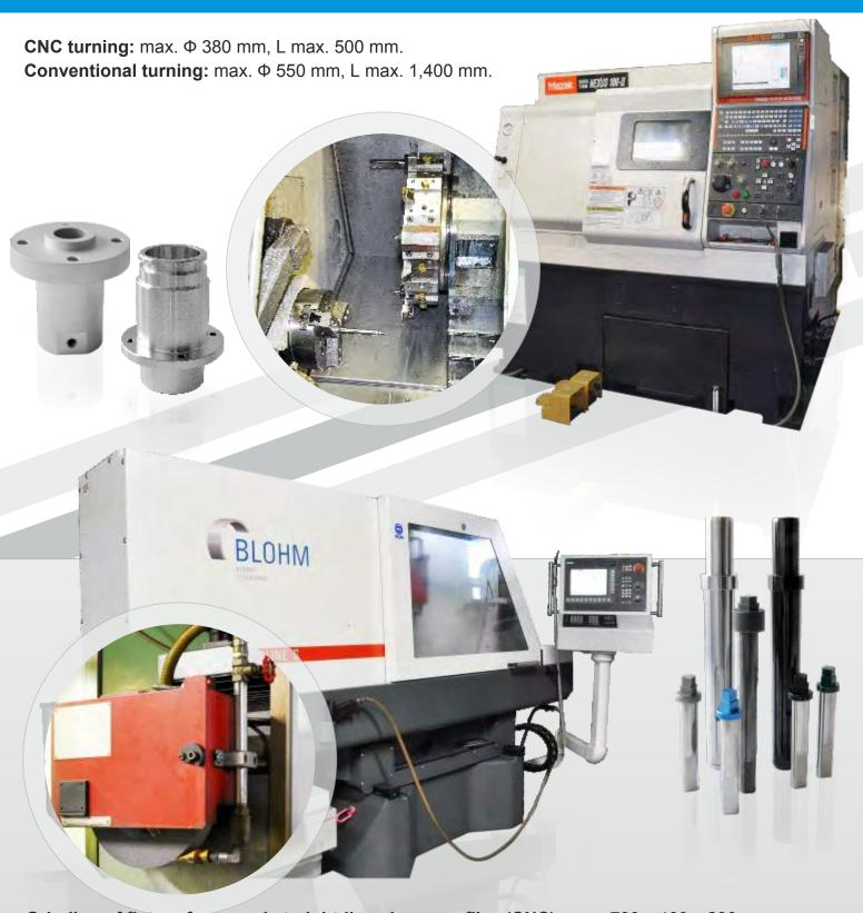
Grinding of flat surfaces and straight-line shape profiles (CNC): max. 700 x 400 x 200 mm. Grinding of rollers: max. Φ 300 mm, L max. 1,000 mm.
